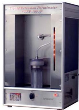
Figure 8. The Liquid Extrusion Porosimeter used in this study.
